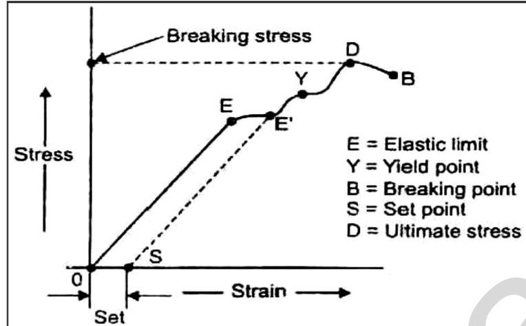
A graph or diagram of stress and strain is shown as above. OE Portion is straight line which indicates that stress is proportional to strain. Therefore the wire obeys Hooke's law upto the point E this point is called elastic limit.
