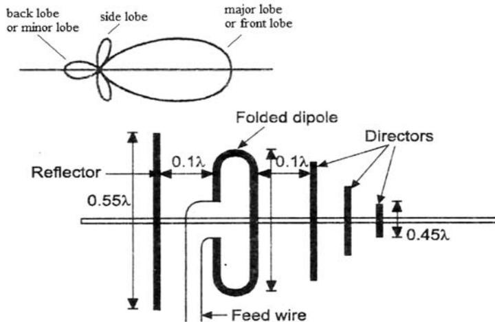
A Yagi-Uda antenna, commonly known as a Yagi antenna, is a directional antenna consisting of multiple parallel elements in a line, usually half-wave dipoles made of metal rods.
