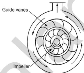
Fig. 1(c) : Casing with guide blades.
