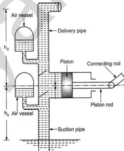
Fig. : Air vessels fitted to reciprocating pump
