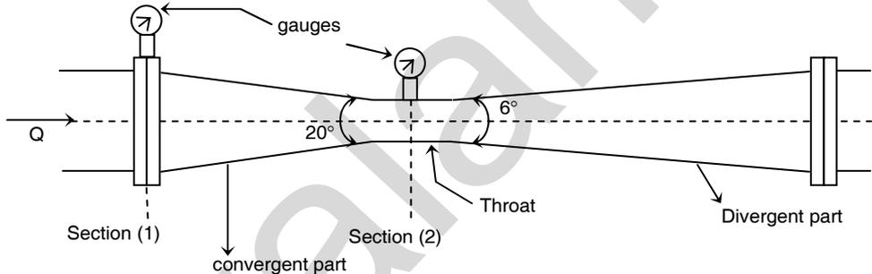
The basic principle on which a venturimeter works is that by reducing the cross sectional area of the flow passage, a pressure difference gives quantity of liquid flowing through the pipe.
