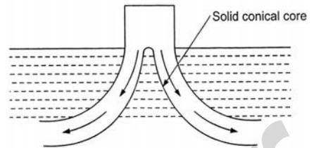
**Fig. 4:** Moody's spreading draft tube of 'Hydrocone'
