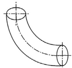
**Fig. 2:** Simple Elbow draft tube.
