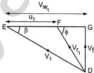
Fig. : changed outlet velocity triangle
