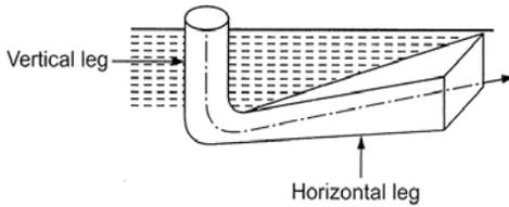
**Fig. 3:** Elbow type draft tube
