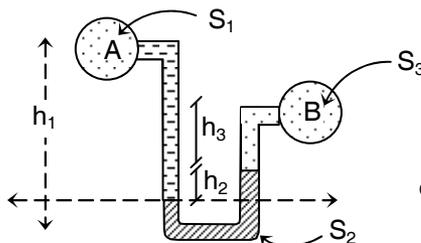
$$\frac{p_A}{w} + h_1s_1 = \frac{p_B}{w} + h_2s_2 + h_3s_3$$
