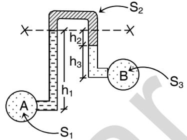
$$\frac{p_A}{w} - h_1 S_1 = \frac{p_B}{w} - h_3 S_3 - h_2 S_2$$
