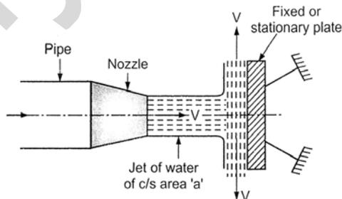
**Fig. :** Direct impact of jet on a stationary flat plate
