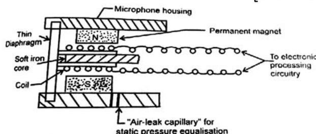
Fig.: Electrodynamic microphone
