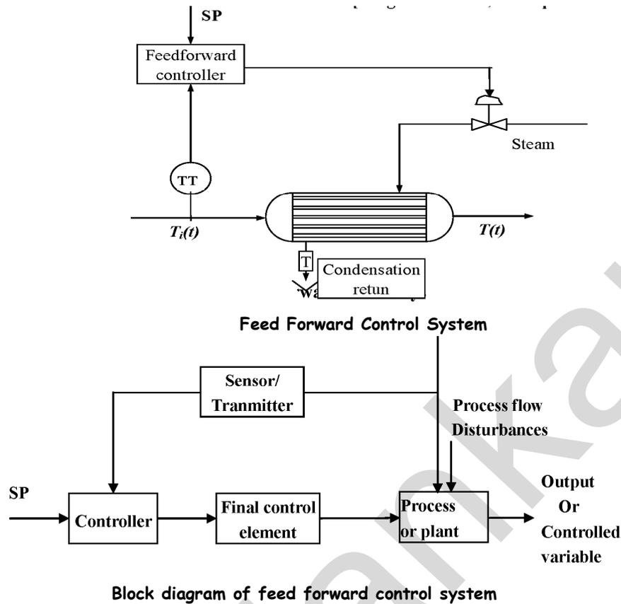
In feed forward control system, disturbances are measured and compensated for them before the controlled variable deviates from set point.
