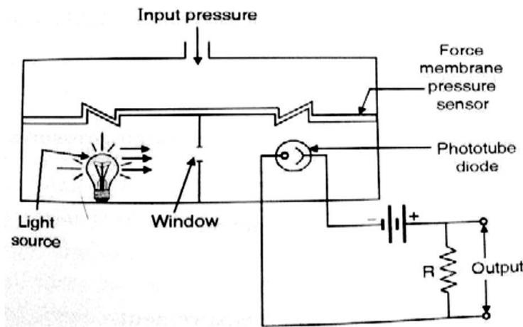
It consists of port for input pressure, pressure sensing member like diaphragm, light source, a small window, a photo tube with output circuit. The function of pressure sensing element is to control the aperture of small window. The amount of output is entirely depends upon the amount of incident light falling on phototube.
