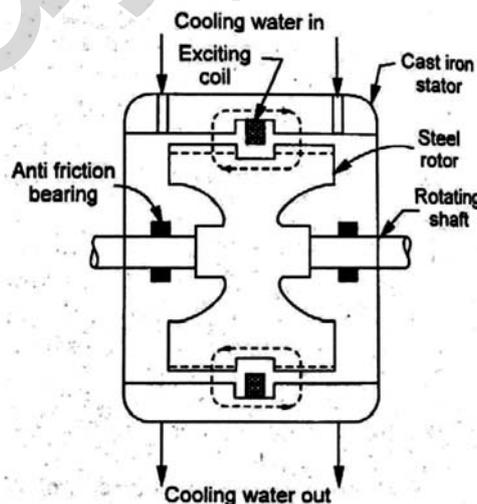
Principle: When an isolated conductor moves through the magnetic flux, voltage is induced and local currents flow in a short circular path (eddy currents) within conductor. These induced eddy currents get dissipated in the form of heat.
