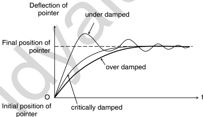
As shown above when critical damping is used pointer takes least time to settle down to the final position and hence critical damping is preferred in all the indicating instruments.
