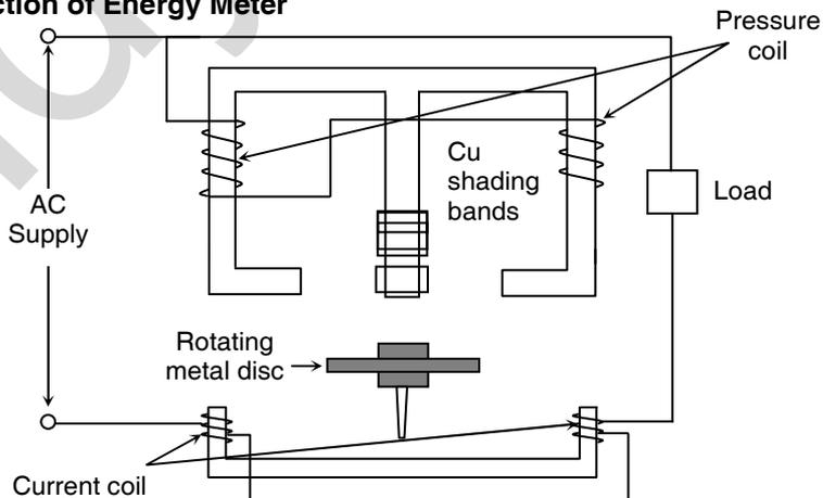
**Application :** Energy meter is basically used for measuring electrical energy consumed by individual flat owner or by Industry. E.E. energy consumed is measured in kilo-watt-hour-which is equal to 1 unit.
