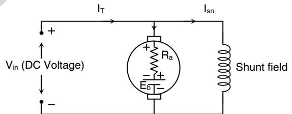
When DC voltage of  $V_{in}$  volts is applied to DC motor total current of  $I_T$  amp starts flowing as shown above. It is divided into two currents.
