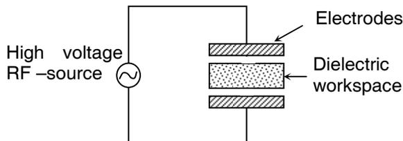
In dielectric heating, a high frequency, high voltage ac voltage is applied across a dielectric material.
