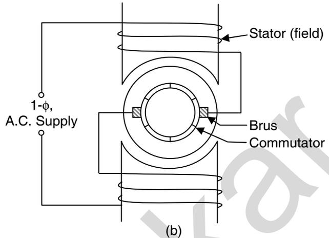
**Reversal of Rotation :** Direction of rotation can be changed by interchanging leads for armature only (i.e. by interchanging leads at brushes) or by interchanging leads for field only.
