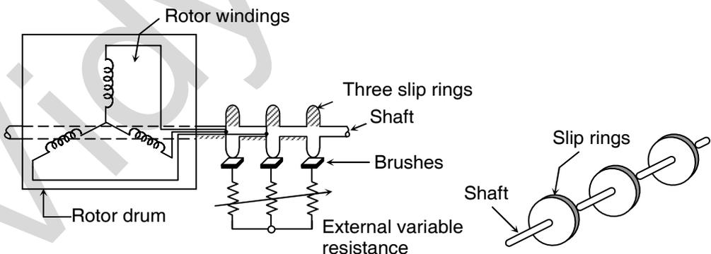
(a) Construction of slip ring rotor or a wound rotor
