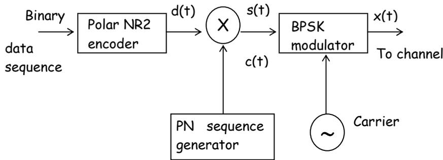
The averaging system reduces the interference by averaging at over a long period. The DSSS system is a averaging system. This technique can be used in practice for transmission of signal over a band pass channel (e.g. satellite channel). For such application the coherent binary phase shift (BPSK) is used in the transmitter and receiver.
