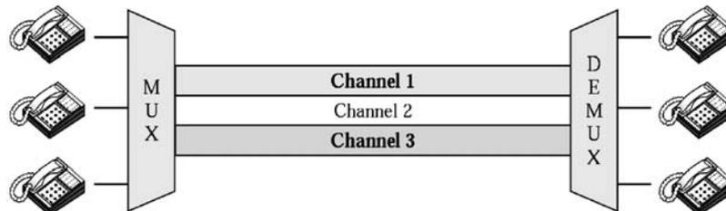
FDM means total range of frequency is divided into number of frequency slots. Each slots of frequency is allotted to each channel. Various channels of different frequencies combined, transmitted through single wire and separated at receiver with the help of De-multiplexer.
