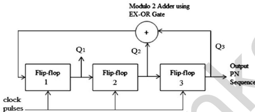
Let initial value of shift register output i.e.  $Q_3 Q_2 Q_1 = 0 0 1$  (any initial value can be taken)
