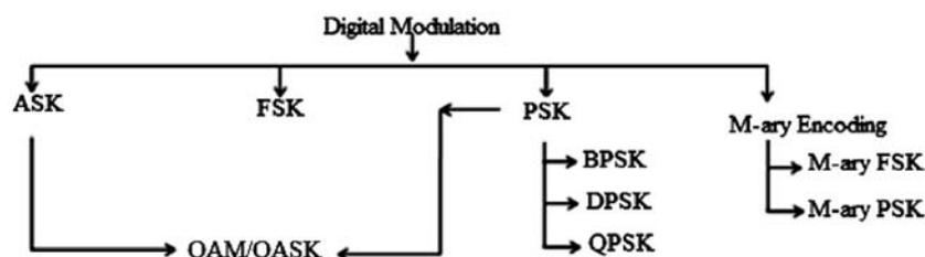
Amplitude Shift Keying (ASK) is the digital modulation technique in which the amplitude of the sinusoidal carrier will take one of the two predetermined values in response to 0 or 1 value of the digital input modulating message signal.
