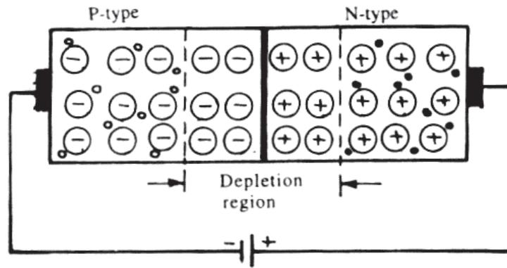
Fig. : Reverse biased P-N junction
