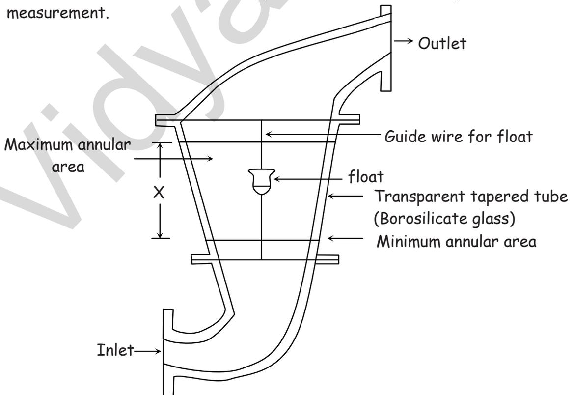
It consists of vertical tapered tube with a float which is free to move in up and down direction. The free area between the float and inside wall of the tube is known as annular orifice. The tube is mounted vertically with a small end at the bottom. The fluid whose flow is to be measured enters the tube from bottom and passes upward around a float and leaves from the top. The venturi tubes are usually made of cast iron or select & are build in several shapes.
