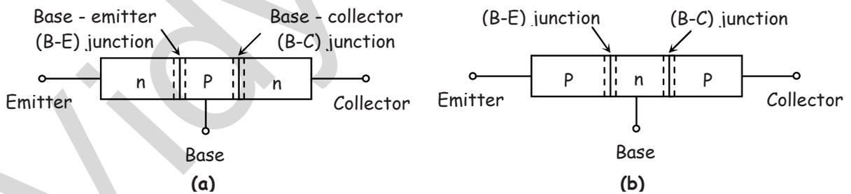
Fig. 1 : Simple geometry of bipolar transistors : (a) npn and (b) pnp
