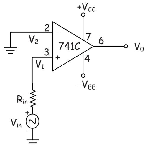
Thus, the output voltage is greater than the input voltage by gain A times and is in phase with the input signal.
