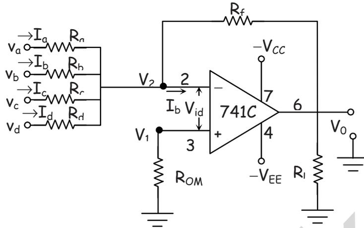
**Scaling Amplifier** : As shown in the above circuit diagram, a number of voltage sources can be connected to the inverting input of op-amp. The value of voltages and resistors can be varied. For an ideal op-amp,
