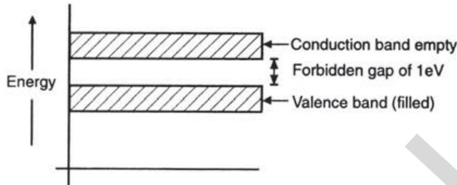
Thus, even heat energy at room temperature is sufficient to lift the electrons from valence band to conduction band. Some electrons jump from valence band to conduction band. Thus, at room temperature, it conducts some electric current. With increase in temperature, width of forbidden energy band is decreased, so that some of the electrons are liberated into the conduction band. In other words, conductivity of semiconductor increases with temperature.
