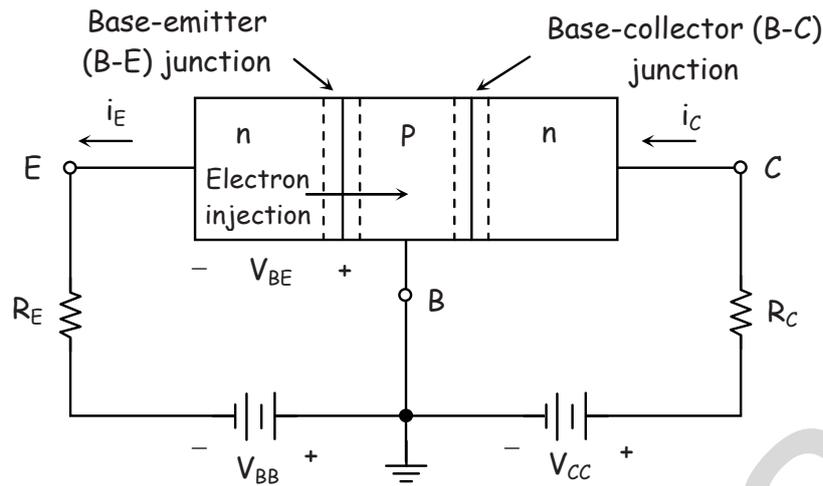
An npn bipolar transistor biased in the forward-active mode.
