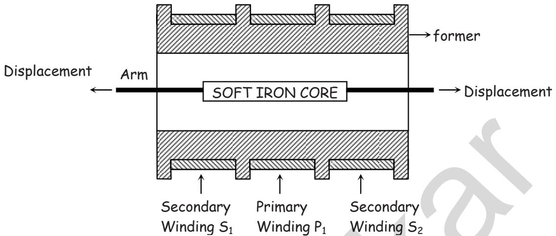
In order to get single o/p voltage 2 secondary winding  $S_1$  &  $S_2$  are connected in series opposition it means the induced voltage of each winding opposes each other. Thus  $e_0 = e_{s_1} - e_{s_2}$
