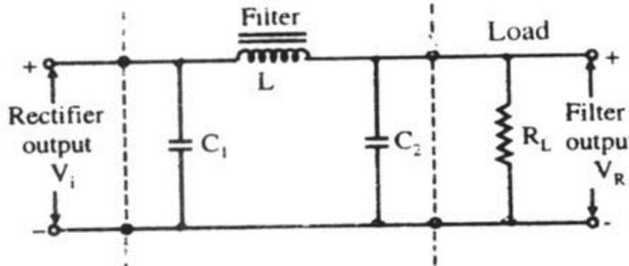
Fig. 1 : Capacitor input filter
