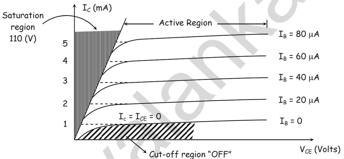
Output characteristics of  $\alpha$  npn transistor in CE configuration
