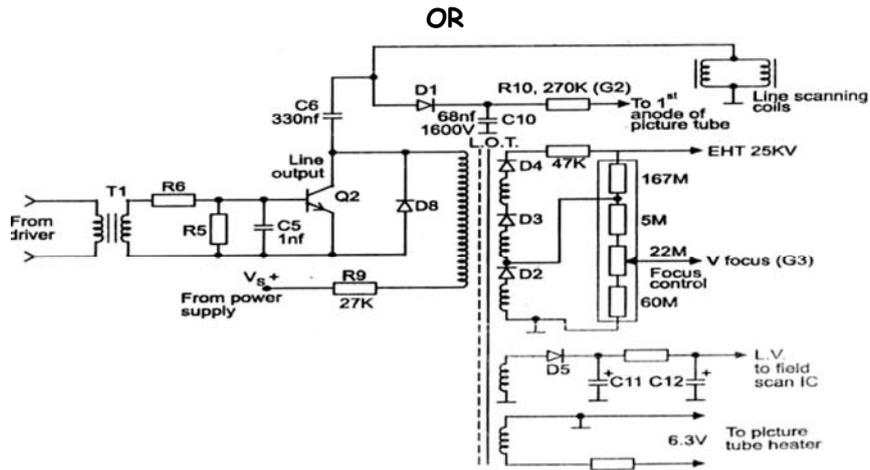
Anode potential (G2) is obtained for screen grid separately at collector of Q2. This is rectified by D1 and then filtered by C10. Output DC voltage is 550 to 800 V. Any failure of G2 means no beam current and hence no spot is produced on screen. Focus anode (G3) potential needed is 6.5kV. It is obtained from diode split winding (D2, D3 and D4). Each stage produces potential of 8kV.
