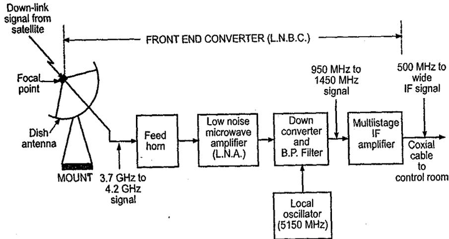
Dish antenna and feed horn: A feed horn is actually a flared open waveguide section which is mounted at focal point and its function is to receive signals reflected towards it by the delivers these to the close by located unit called as Low Noise Block Converter (LNBC).
