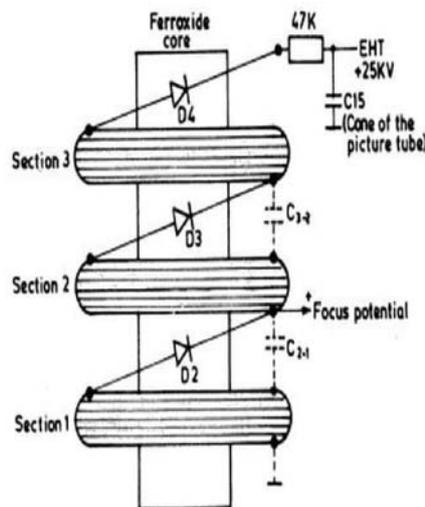
principle of split-diode addition to obtain EHT and focus anode potentials for a colour picture tube.
