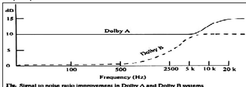
**Fig. Signal to noise ratio improvement in Dolby A and Dolby B systems**
