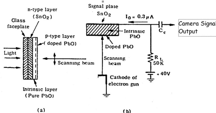
Fig. 1 : Plumbicon camera (a) target details (b) Output signal current
