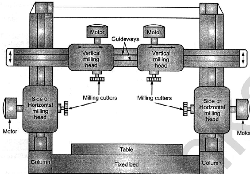
Fig. 1 : Planer type Milling Machine (Block diagram)
