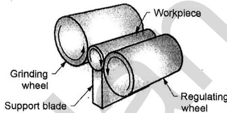
**Principle of centreless grinding**
