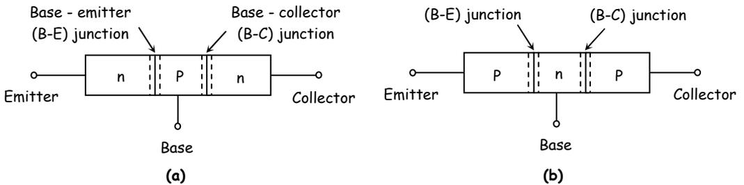
Fig. : Simple geometry of bipolar transistors : (a) npn and (b) pnp
