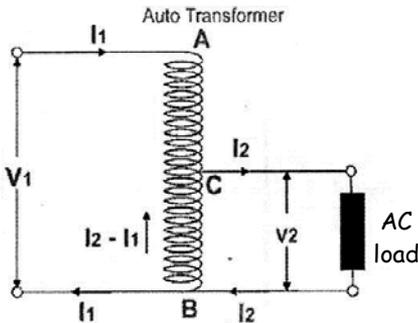
Fig. 1: Step Down auto transformer
