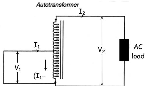
Fig. 2: Step Up auto transformer
