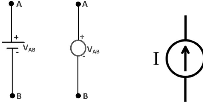
A current source is an electronic circuit that delivers or absorbs an electric current which is independent of the voltage across it.
