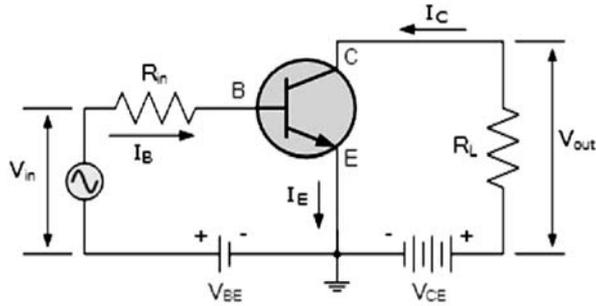
In this type of configuration, the current flowing out of the transistor must be equal to the currents flowing into the transistor as the emitter current is given as  $I_E = I_C + I_B$ .
