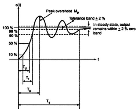
Fig- Unit step response of second order system
