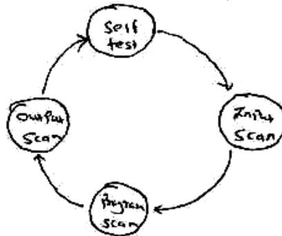
**Speed of execution:** The speed at which PLC scans memory and executes the program is referred as a speed of execution. Higher CPU speeds provide faster performance that shortens task time.
