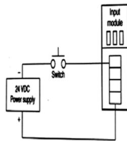
fig 1-Sourcing D.C input module with a sinking switch
