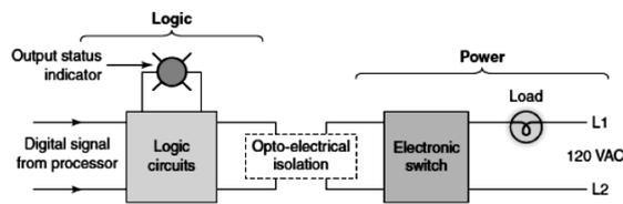
Fig- Output module of PLC
