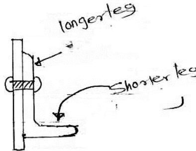
In the shorter leg is connected to gusset plate, then the bending stress induced in the section is large due to outstanding longer leg, because of which the stress distribution in the section is non-uniform and hence it may lead to fracture of the member prematurely.
