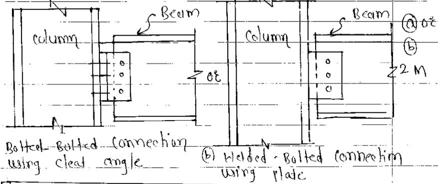
Fig: Beam to column connection
