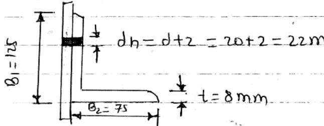
$$T_{dn} = \alpha A_n \frac{f_u}{r_{m1}}$$
