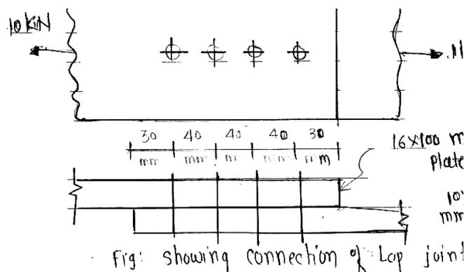
Q.1(b) (ii) Draw neat sketches of bolted connections in case of :
