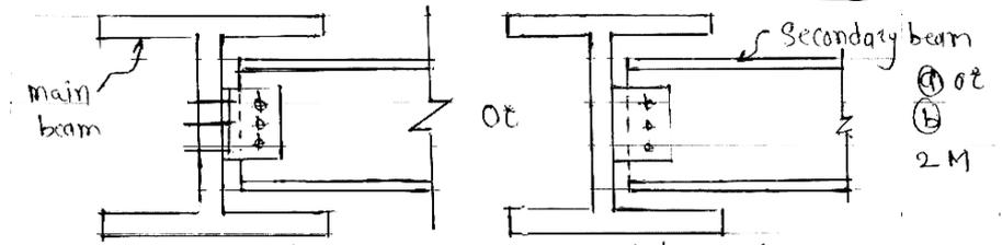
Fig: Beam to Beam Connection When flanges are not at same level
