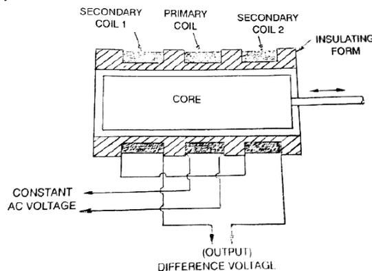
**Explanation:** LVDT works on mutual inductance principle. It is a transformer consisting of three symmetrically spaced coils carefully wound on an insulated bobbin. It consists of a primary coil wound on an insulated bobbin and two identical secondaries symmetrically spaced from the primary. AC carried excitation is applied to the primary and two secondaries are connected externally in a series opposition circuit. There is noncontacting
