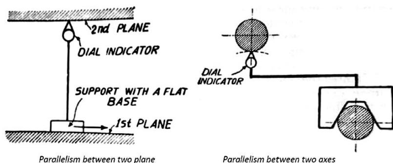
**Parallelism between two planes:** The test for parallelism of two planes is carried out in two directions (generally perpendicular to each other). The dial indicator, which is held on a support with a flat base, is moved in one plane over a given length, and the feeler is made to rest against the second plane; and the deviation is noted down.
