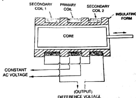
**Explanation:** LVDT works on mutual inductance principle. It is a transformer consisting of three symmetrically spaced coils carefully wound on an insulated bobbin. It consists of a
