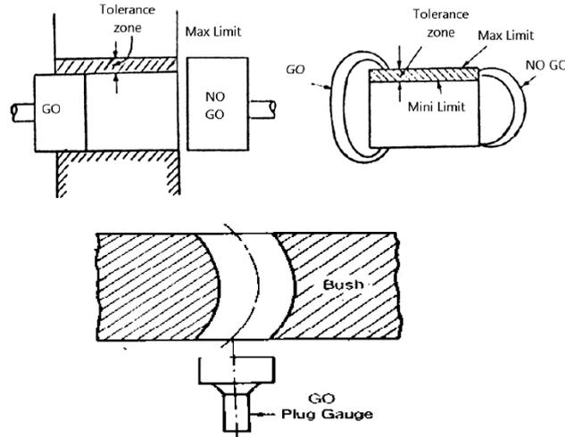
Fig.: Checking a bush with curved
