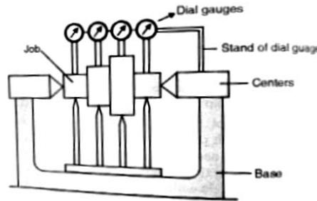
**Explanation:** Multi Gauging machines are useful for measurement of number of dimensions at a time. Part to be checked are compared with setting standards and the deviation is recorded.
