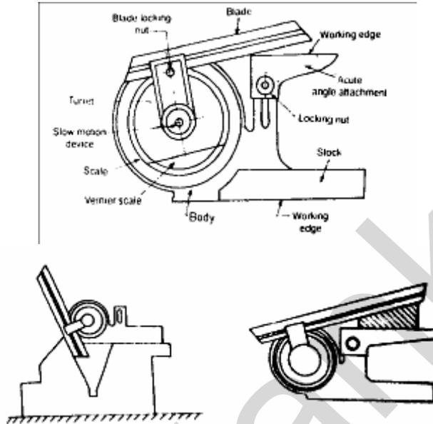
Use of bevel protector for checking of V block and measuring acute angle
