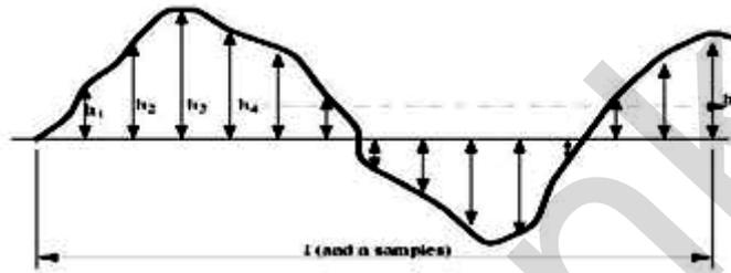
$R_z$  : in this the average difference between the five highest peaks and five deepest valleys within the sampling length, measured from a centre line.
