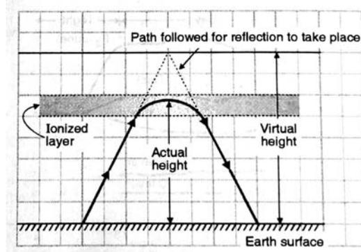
**Fig.:** Virtual height of an ionized layer
