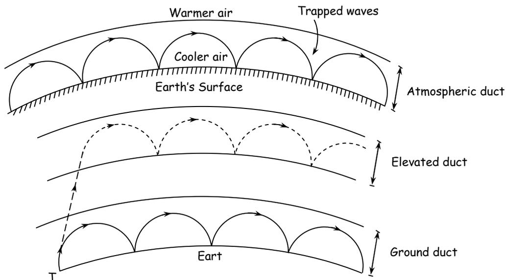
As the height above the Earth increases, the air density decreases and refractive index increases. The change in refractive index is normally linear and gradual but under certain atmospheric condition a layer of warm air may be get trapped above the cooler air, often over the surface of water, due to this refractive index will decreases rapidly with height than usual. (This happens near the ground, often within 30 m) Due to this rapid reduction of refractive index, the microwaves will completely
