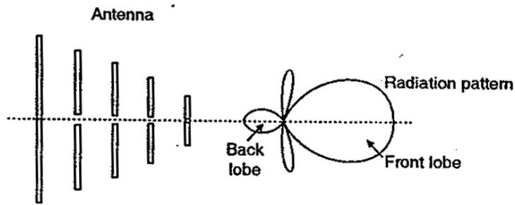
Fig. 2 : Radiation pattern of Yagi-antenna.
