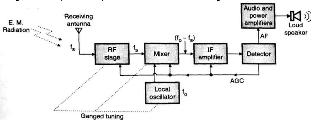
Fig.: The superheterodyne receiver
