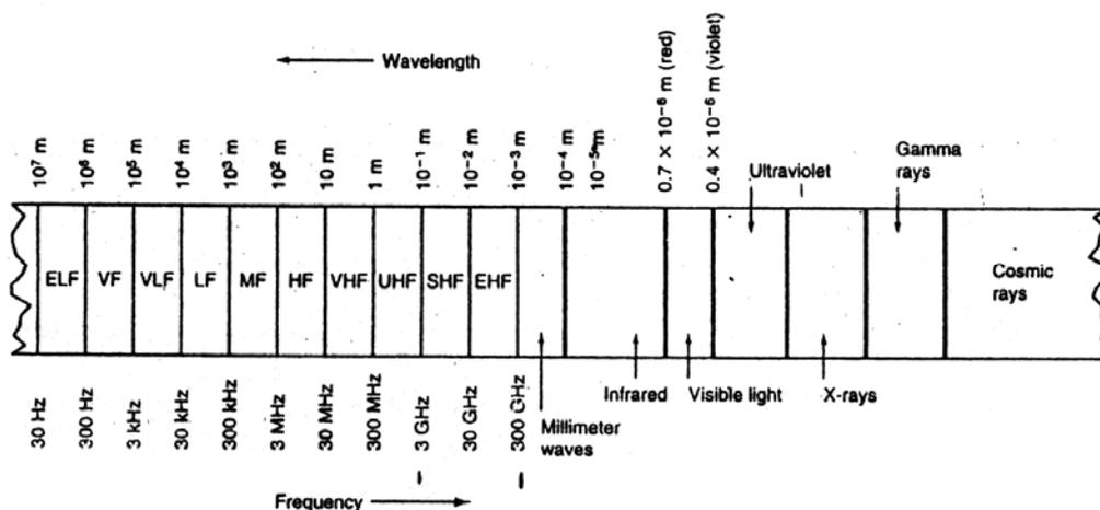
**Fig. :** The electromagnetic spectrum used in electronic
