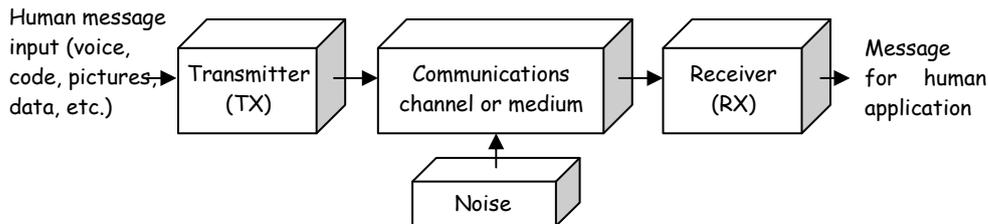
Fig.1: The basic elements of any communications system.
