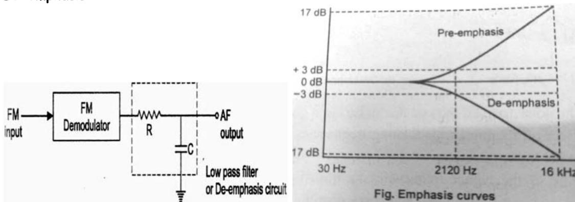
In FM, noise has greater effect on higher modulating frequencies than the lower one. Therefore the higher modulating frequencies have to be boosted artificially at the transmitter before modulation and corresponding cut off at the receiver after demodulation.
