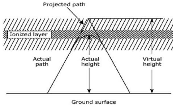
The incident and refracted rays follow paths that are exactly the same as they would have been if reflection had taken place from a surface located at a greater height called virtual height of this layer.
