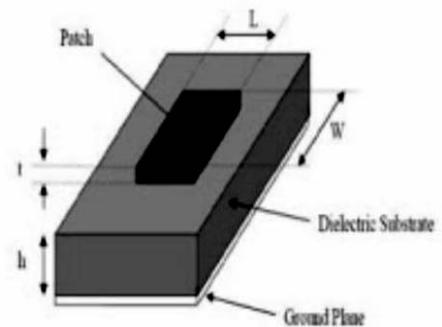
Structure of a Microstrip Patch Antenna
