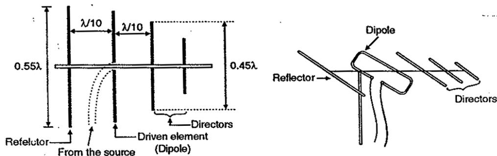
**Fig. 1 : Construction of Yagi antenna.**
