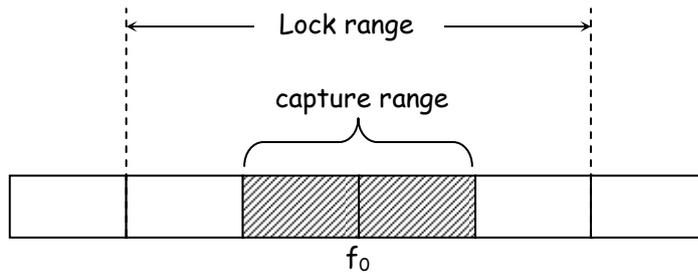
In locked phase, the voltage controlled oscillator output will be equal to the input signal and error signal will be identified to the original modulating signal of the frequency modulator input.
